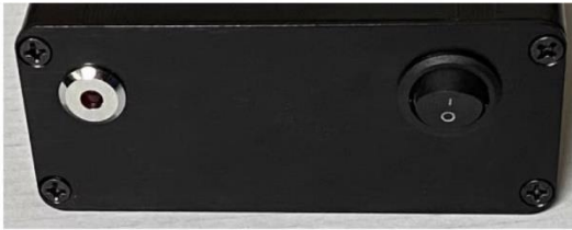
前面板手动开关, LED 电源灯
